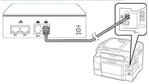
3. Plug Network Port 1 into your local network that has access to the internet. This is needed to send and receive faxes. Network Port 2 is set up as a bridge from Network Port 1 to allow you to have Port 2 act as a passthrough switch to let you plug in another device such as a PC or anything else that needs network and where you only have a single network drop.
